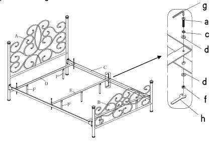
**Step 3 :** Attach each Metal Support Leg (F) to Metal Slats (D & E), using Bolt (b), Flat Washer (d), tighten by hand at first, securely tighten with Allen Wrench (g), but do not over tighten See **Figure 3**
