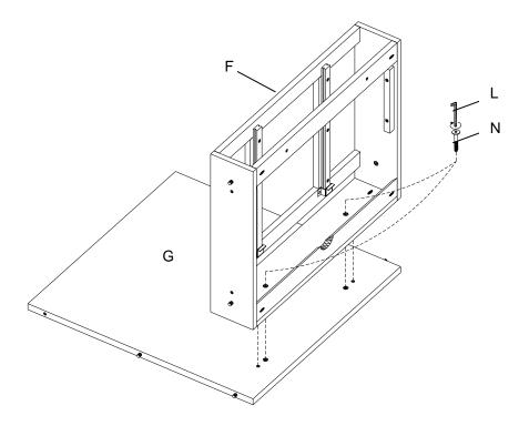
3. Align the dowels from the Desk Center assembly (F) to the Desk 3 Drawer (E) on the right side, and Desk 1 Drawer (D) on left side. Secure using bolts (N) and tighten with Allen key (L)
