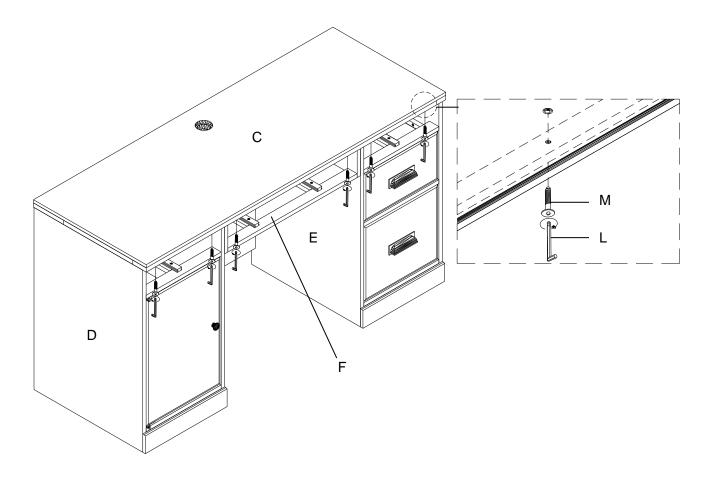
7. Re-install the drawers to the cases that were taken out earlier. Place the wood grommet (H) to close the wire management hole.
