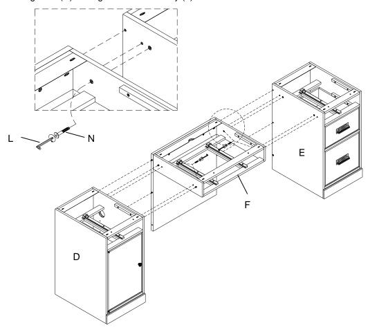
4. Secure the back panel (G) to Desk 1 Drawer (D) and Desk 3 Drawer (E) by attaching the bolts (U), lock washer (O), and half moon washer (R). Tighten using Allen key (L)
