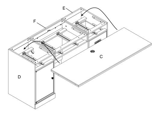
6. Secure the desk top (C) by Aligning the pre-drilled holes in the top rails of the desk assembly (D,E,F) with the holes on the underside of the Desk Top (C). Secure using bolts (M) and tighten with Allen key (L)
