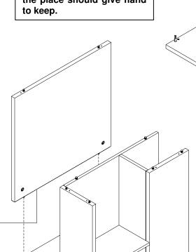
8. Attach the Large Side Panel (C) on the Top Panel (A). Align the dowels on the side with pre-drilled holes on top.
