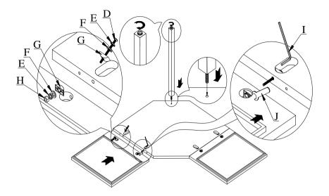
8. Put the Pedestals (K) in the position as shown. Two people turn the connected top right side up and lift to the desired height. Make sure the two Pedestals (K) align with the positioning frames underneath the top and slowly lower the top down until it sits firmly on the Pedestals (K). Adjust the recessed levelers underneath the Supporting Leg (N) and Pedestal legs to make sure the whole assembly is balanced.
