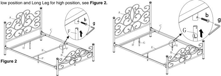
**Step 3:** Attach Metal Slats (D) with Support legs attached, to Side Rail (C) using Bolts (a), Spring Washers (c), Flat Washers (d) and Nuts (f), tighten by hand at first, securely tighten with Allen Wrench (g) and Wrench (h), but do not
