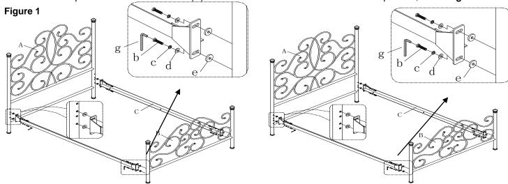
**Step 2:** Attach each Short Support Leg (F) or Long Support Leg (G) to Metal Slats (D & E), using Bolt (b), Flat Washer (d), tighten by hand at first, securely tighten with Allen Wrench (g), but do not over tighten. Please note Short Leg for
