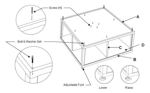
7. Adjust the adjustable levelers on the bottom of the feet by loosening or tightening them, as needed, so it sits evenly on the floor. See above illustrations.
