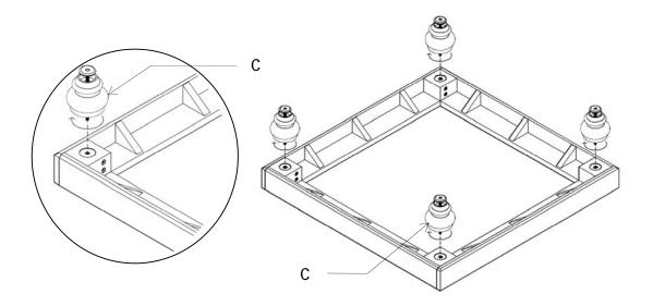
4. Place the assembled Cushy Turned Wood Base in an upright position. Adjust the adjustable levelers on the bottom of the Turned Legs (C), as needed so the piece sits evenly on the floor. **See illustrations below.**
