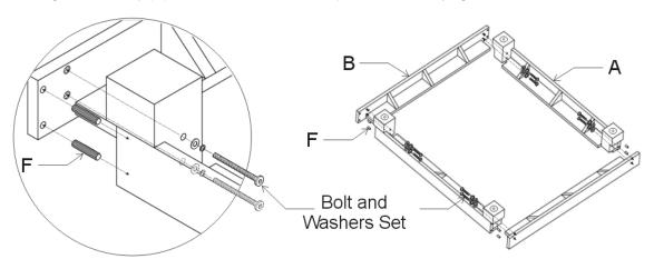
3. Place the assembled Cushy Pedestal Base in an upright position. Adjust the adjustable levelers on the bottom of the feet, as needed. See illustration.
