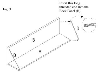
Step 4: Secure the two ends of each Wire Rod (D) with a Flat Washer (E) and a Pan-Head Nut (F) from behind and under the shelf by using a Phillips Head Screwdriver.
